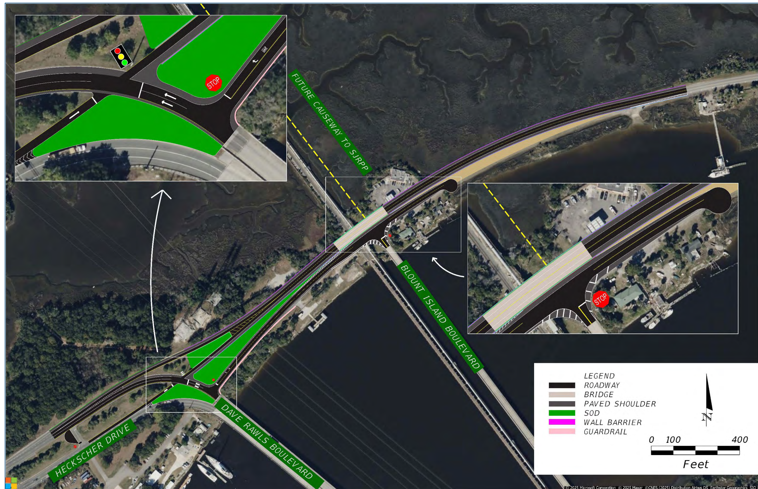
Figure 17 – Single Grade Separation
