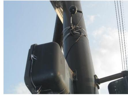
**Pedestrian detection sensor (FLIR™) installed at the SR 13 and Haley Road Intersection in Jacksonville.**
